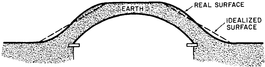
Figure 6.111. Configuration of mounded arch.
